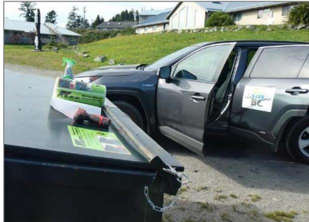
**Figure 25. Installing chains with carabiners and instructional decals on Hitacu bins**
